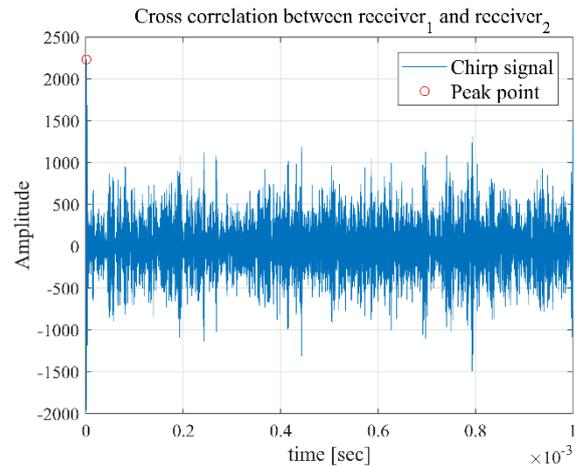
**Figure 8 – Correlation result of two received signals for Chirp**
