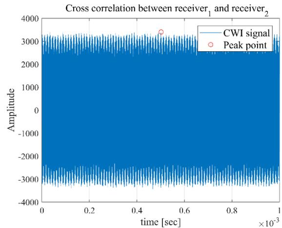
Figure 4 – Correlation result of two received signals for CWI
