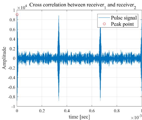
**Figure 7 – Correlation result of two received signals for pulse**
