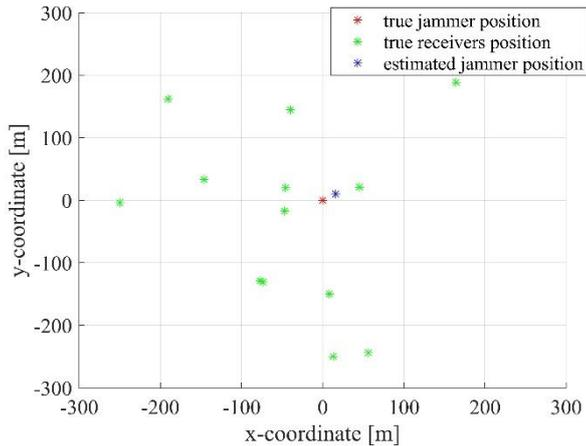
**Figure 9 – The results of jammer position estimation by using proposed method**
