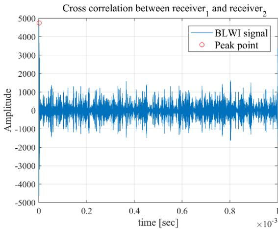
**Figure 6 – Correlation result of two received signals for BLWI**
