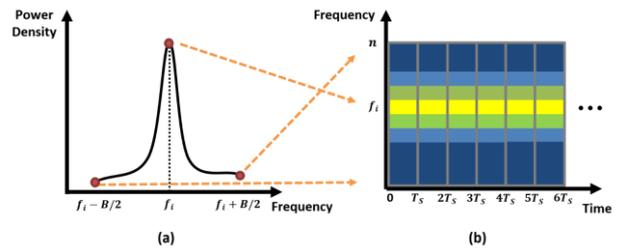
**Figure 3 – Method of generating a 2-D image in the time-frequency domain for a single receiver. (a) PSD of n sample length IF signal at any one time (b) Generated 2-D image**
