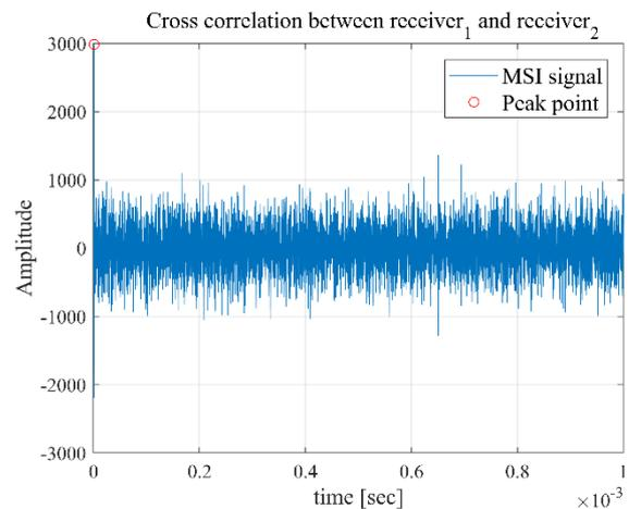
Figure 5 – Correlation result of two received signals for MSI
