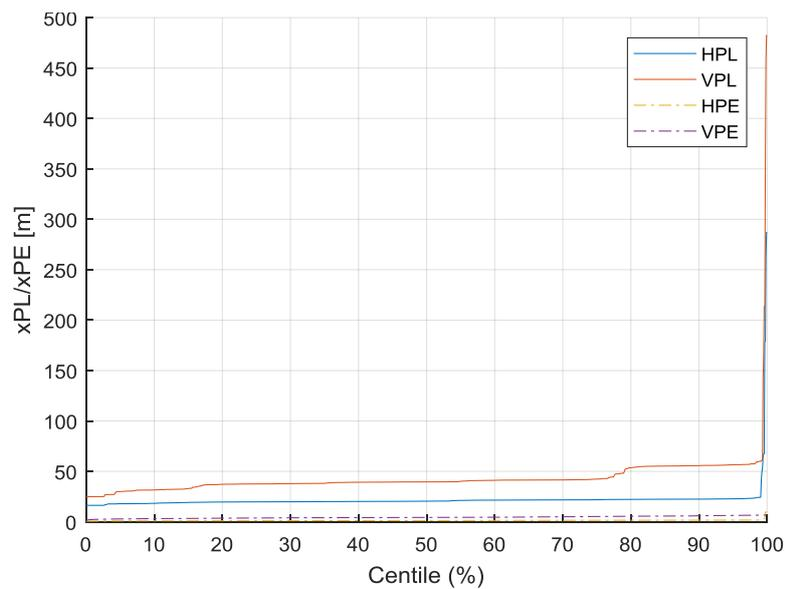
**Figure 5: Example of error and protection level distributions in the Railway environment.**
